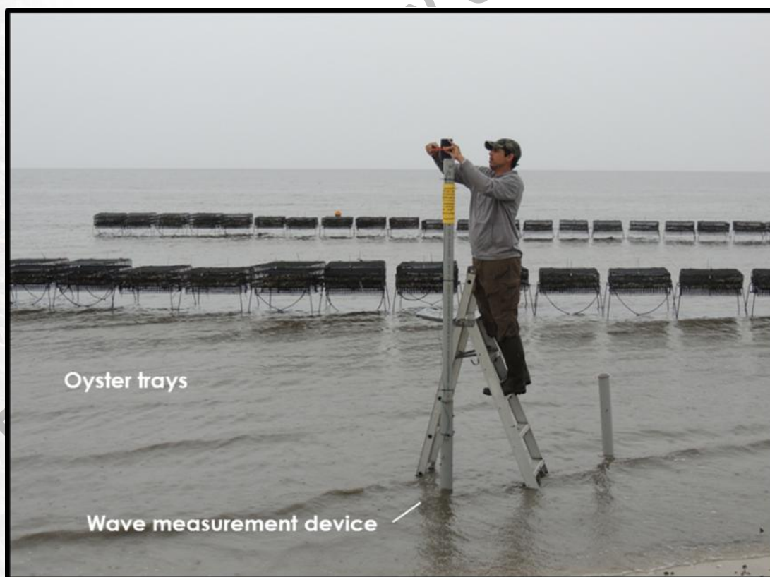
Figure 21. A double row of oyster racks proved the most effective method of wave-attenuation tested.
